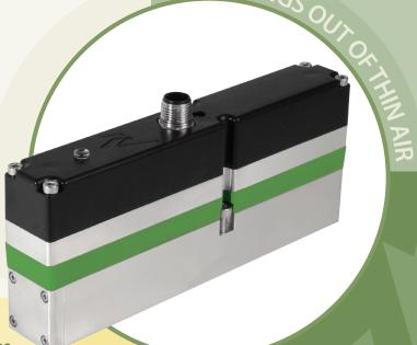
Nexmatix's new energy efficient ISO valves use on average 20-40% less compressed air than conventional directional control valves. The valves perform like conventional valves but use a unique spool configuration and on-board microelectronics to recycle compressed air. All valves conform to international standards 15407-1 and 15407-2.
