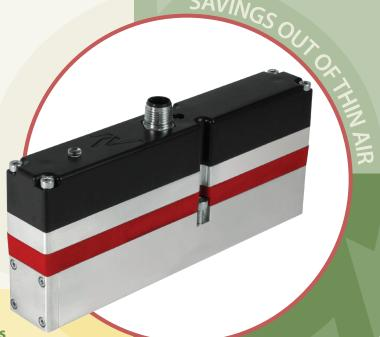
**Nexmatix's new energy efficient ISO valves** use on average 20-40% less compressed air than conventional directional control valves. The valves perform like conventional valves but use a unique spool configuration and on-board microelectronics to recycle compressed air. All valves conform to international standards 15407-1 and 15407-2.
